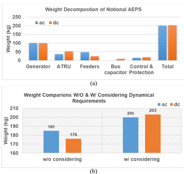
Fig. 21. Estimated system weight: (a) weight decomposition of notional Aircraft EPS and (b) weight comparisons.
