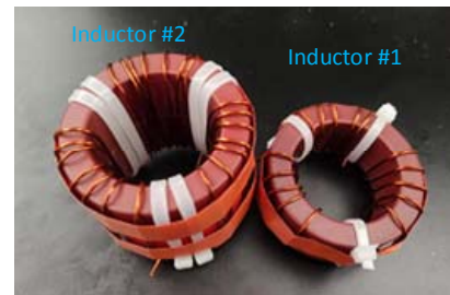
Fig. 8. The prototypes of two CM inductors.
