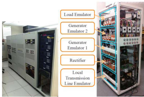
Fig. 12. CURENT Hardware Testbed (HTB).
