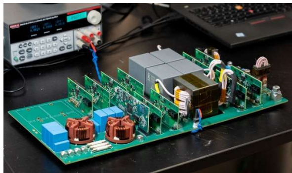
Fig. 9 Prototype of 11kW+3.5kW integrated charger with PFC
