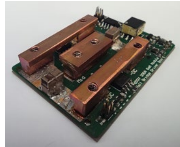
Packaged GaN Module (45*33*9.6 mm 3 )
