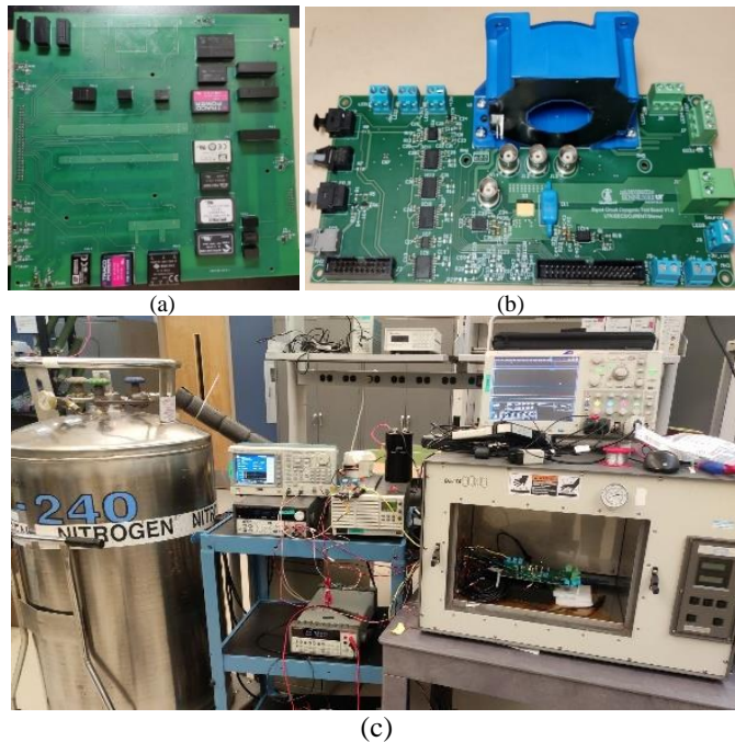
Fig. 1. Developed test setup: (a) APS test board, (b) isolator, fiber optics, and isolation amplifier test board, (c) cryogenic test chamber with liquid Nitrogen cylinder.
