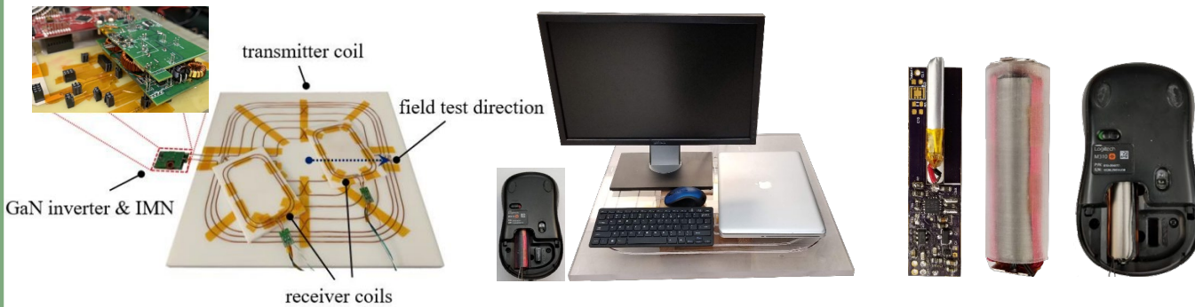
Multi-receiver 100 W workstation with 92% end-to-end efficiency
