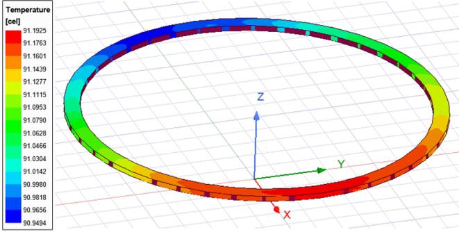
Fig. 2. Thermal simulation of Rx coil in Ansys Icepak.
