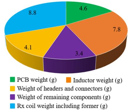
Fig. 11. Weight breakdown of the receiver.
