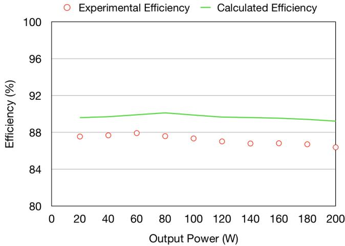
Fig. 12. Measured and calculated dc-dc prototype efficiency.
