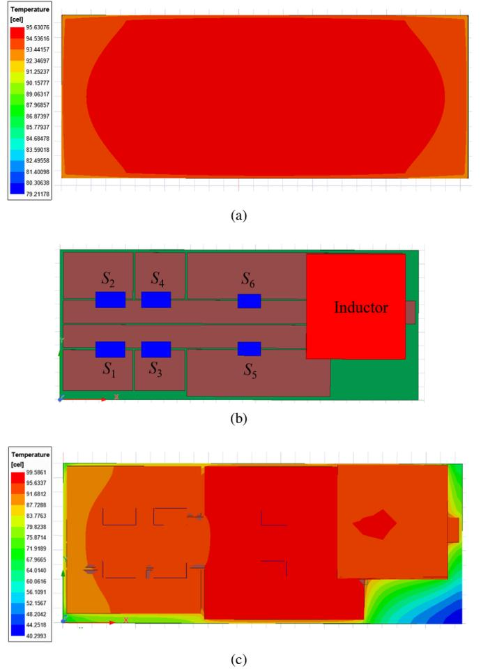
Fig. 5. Ansys Icepak thermal simulation result for power stage models at varying fidelity. (a) Total power stage loss applied to a  $70 \times 29$  mm copper plane on the top layer of a PCB. (b) Layout diagram of PCB design for prototype, and (c) Icepak thermal simulation of detailed PCB layout.
