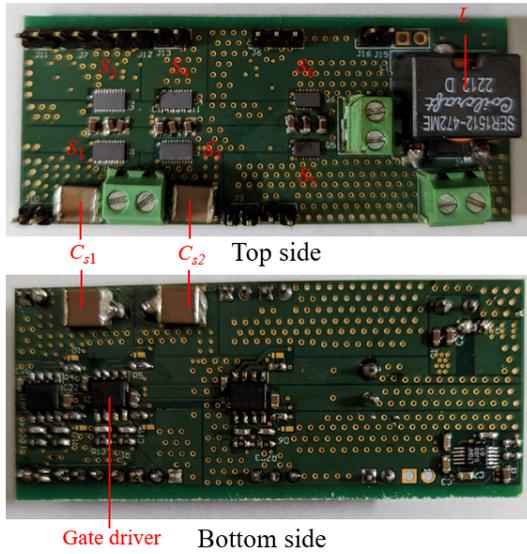
Fig. 6. Photograph of the receiver power stage.
