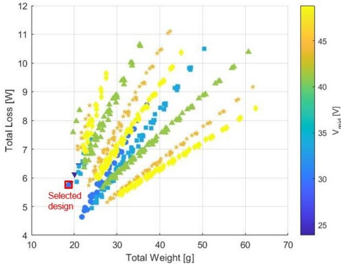
Fig. 4. Design space for system-level optimization of receiver.
