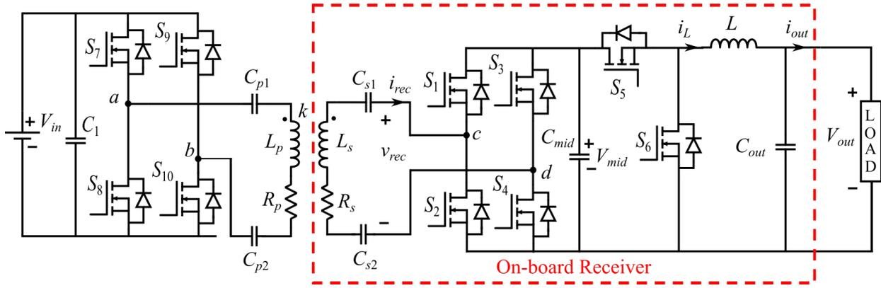
Fig. 1. Circuit schematic of the WPT system, including inverter, Tx and Rx coils, rectifier, and buck.
