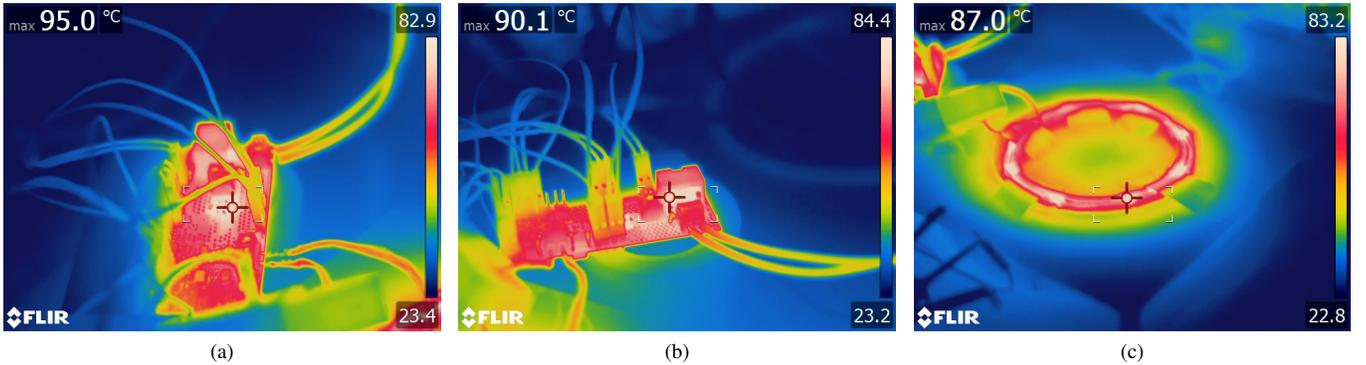
Fig. 10. Thermal photographs at full power: (a) power stage thermal image focusing on the FETs, (b) power stage thermal image focusing on the inductor, and (c) thermal image of coils.
