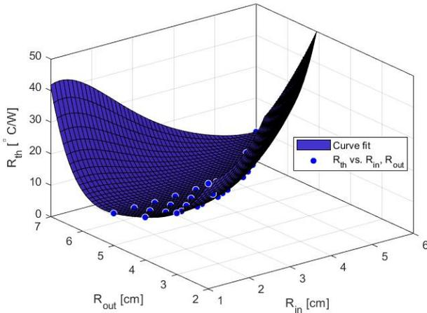
Fig. 3. Curve fitting of coil thermal Resistance for varying coil inner and outer radii, based on Ansys Icepak simulation results.
