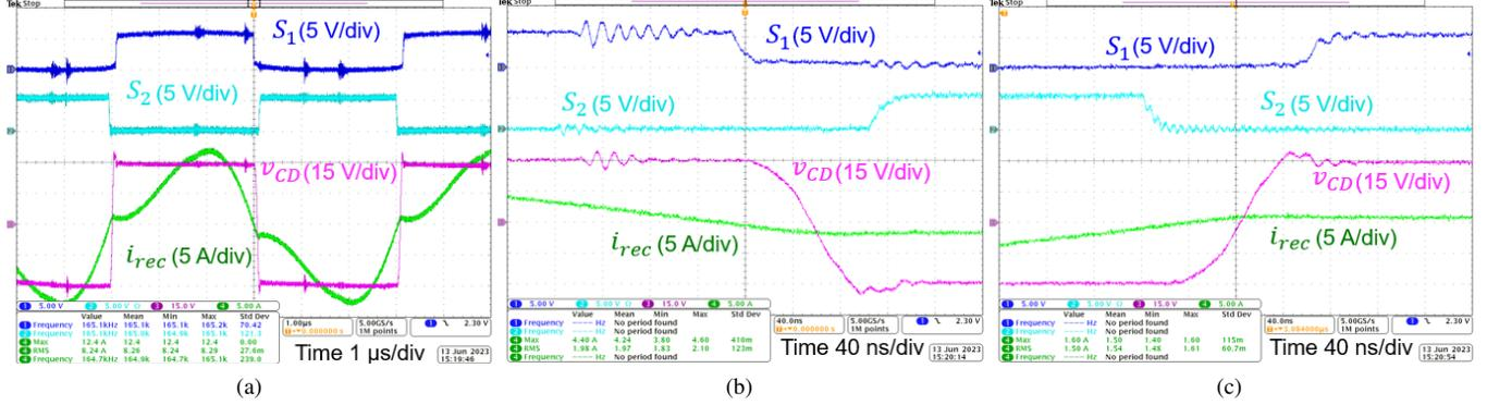
Fig. 9. Gate pulses,  $i_{rec}$  and  $v_{cd}$  of the rectifier at 200 W: (a) one full period, (b) zoomed-in view of  $S_1$  going low and  $S_2$  going high transition, and (c) zoomed-in view of  $S_1$  going high and  $S_2$  going low transition.
