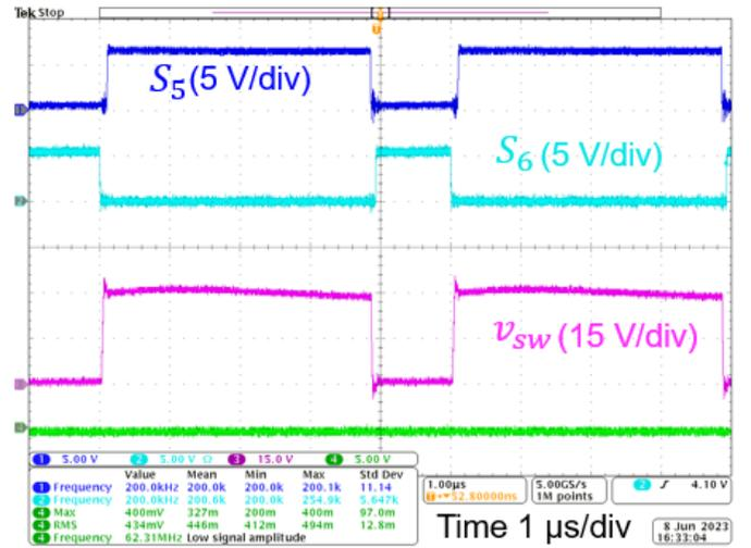
Fig. 8. Gate pulses and switch node voltage  $v_{sw}$  of the buck at 200 W for one full period.
