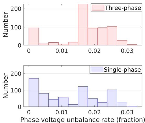
Fig. 8: Histogram of maximum voltage unbalances for the feeder.
