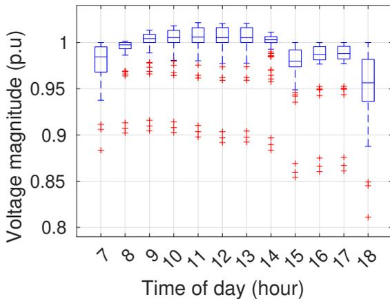
Fig. 6: Voltages boxplots for single-phase regulation case.
