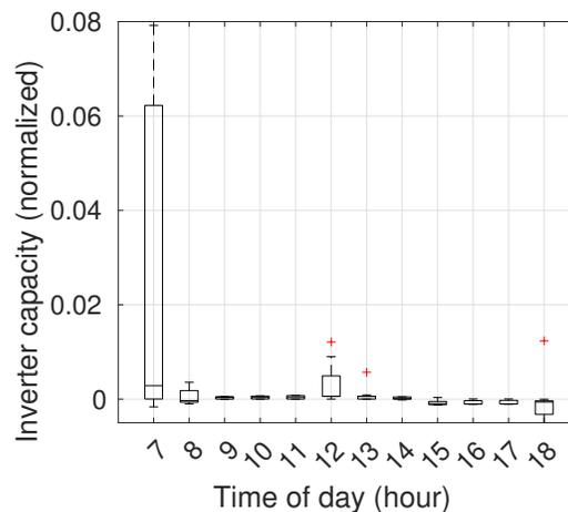
Fig. 10: Boxplots of capability usage differences between three-phase Volt/Var and single-phase Volt/Var scenarios.
