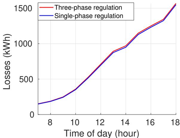
Fig. 11: Integrated losses on the feeder cables, for each batch of simulations.
