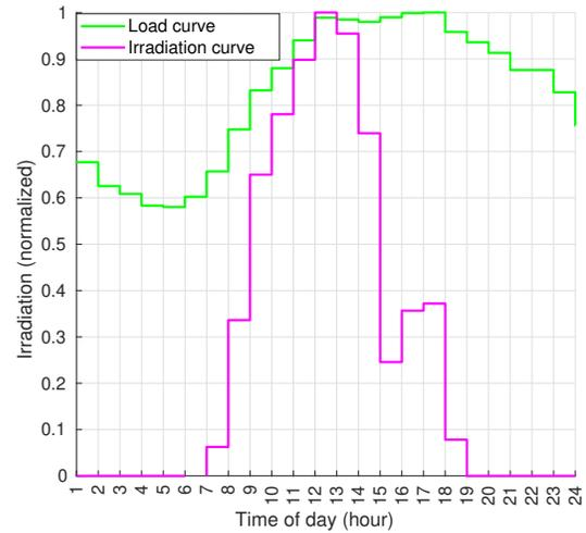
Fig. 4: Load and solar irradiation curves considered in the two executed daily simulations.
