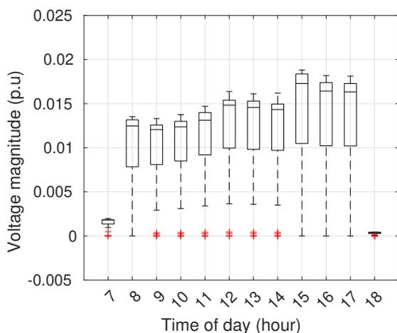
Fig. 9: Boxplots of the differences between the buses phase voltage unbalance rates of the three-phase and single-phase cases.
