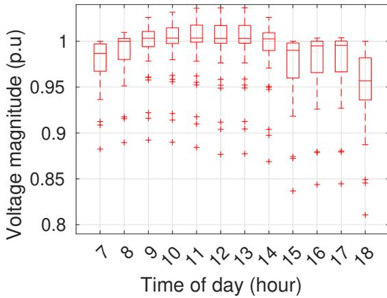
Fig. 5: Voltages boxplots for three-phase regulation case.
