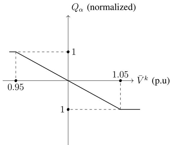
Fig. 3: Configured Volt/Var characteristic curve for inverters in executed simulations.
