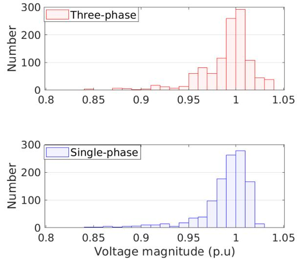
Fig. 7: Histogram of phase-neutral node voltages between 7:00 and 19:00.
