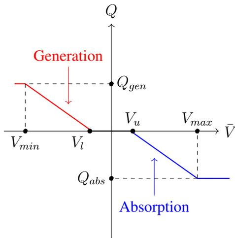
Fig. 1: Generic Volt/Var characteristic curve.
