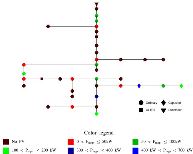
Fig. 2: Map of photovoltaic systems placement and sizing on IEEE 34-Bus test case.
