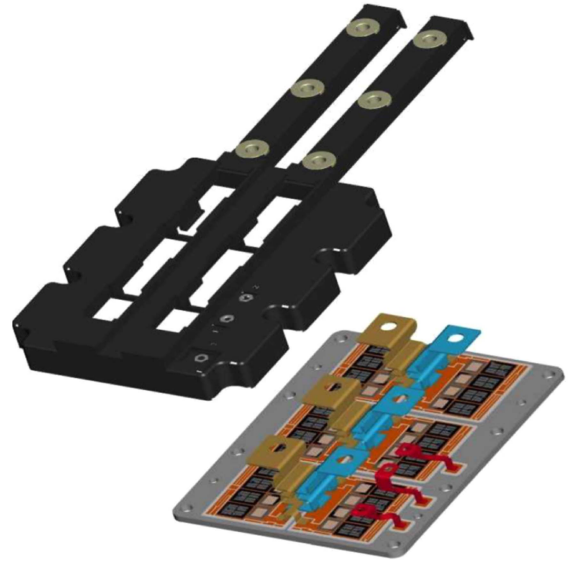
Fig. 11. Infineon IHM/IHV B module package and internal layout [39].
