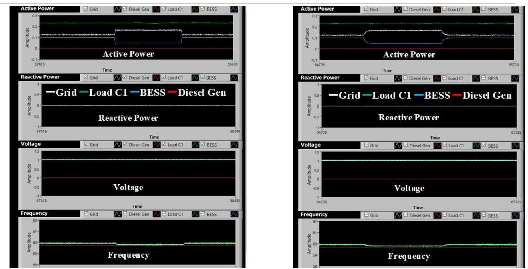
Fig. 4. Inverter response during active power command changing: (a) K_p = 0.05 and K_i = 0.0025 , (b) K_p = 0.01 and K_i = 0.0025
