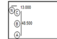
345 kV line spacing
