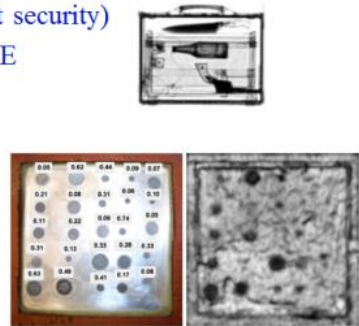
NASA Shuttle tile corrosion experiment
