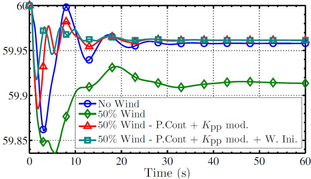
Figure 3 (left): Frequency response of 10-machine New England System with 50% wind penetration, showing improved frequency regulation using wind turbine blade pitch control.
