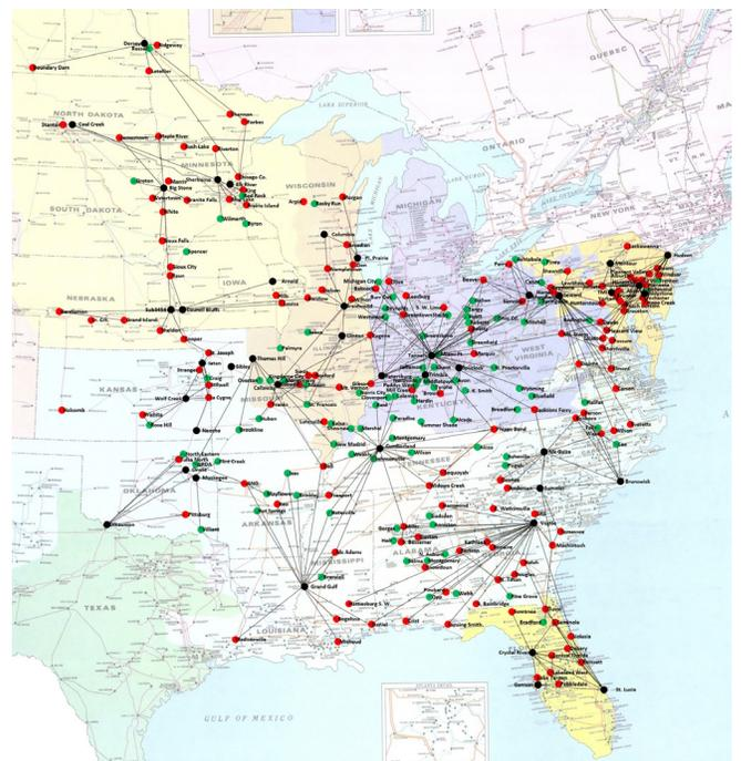
Figure 1: Reduced US Eastern Interconnection Model
