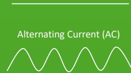
Figure C2.1 AC vs. DC frequency waves. Alternating current most commonly reveals a waveform known as a sine wave, due to the voltage (the force interacting with current) and current alternating.
