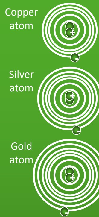
Figure E1.1. The internal structure of three common conductors copper, silver, and gold. Conductors have an internal structure that allows free electrons to flow. They normally have 1-3 valence electrons in their outermost orbital shell. With fewer electrons, they are less resistant to the flow of current.
