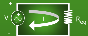
Figure B3.3. A simple circuit schematic. In this circuit, I , or current, travels from high to low voltage, clockwise starting from the positive terminal of the battery through R where it returns to the negative terminal of the battery. See Table B1.4 for a key to the circuit symbol diagrams (Appendix p. 183).
