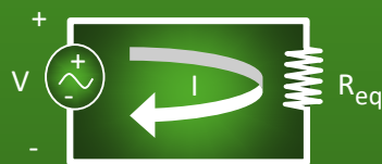
Figure B2.3. A simple circuit schematic. In this circuit, I , or current, travels from high to low voltage, clockwise starting from the positive terminal of the battery through R where it returns to the negative terminal of the battery. See Table B1.4 for a key to the circuit symbol diagrams (Appendix p. 183).
