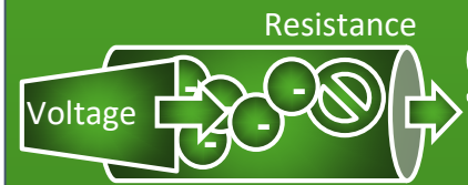
Figure A6.2 Voltage, current, and resistance within a conductor (wire). You can see that the resistance is an obstacle in the way of the flow of electrons (current).
